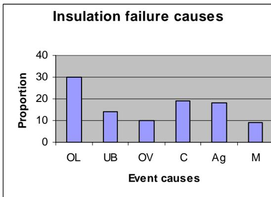
Fig.2 Insulation failure initiating causes distribution
