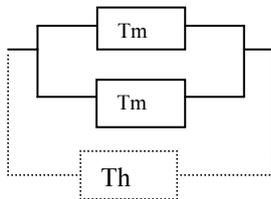
Fig.9 Redundancy at thermal sensor circuit
