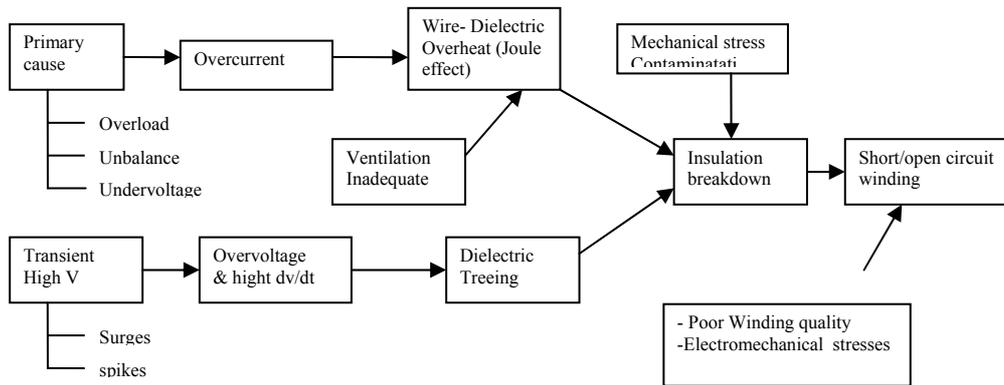
Fig 1 Failure mechanisms sequence of the electrical stator windings
