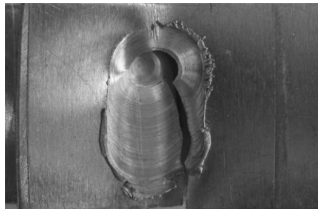
Fig. 9 – Partially curved interfacial fracture mode that is caused by high level of plunging depth.
