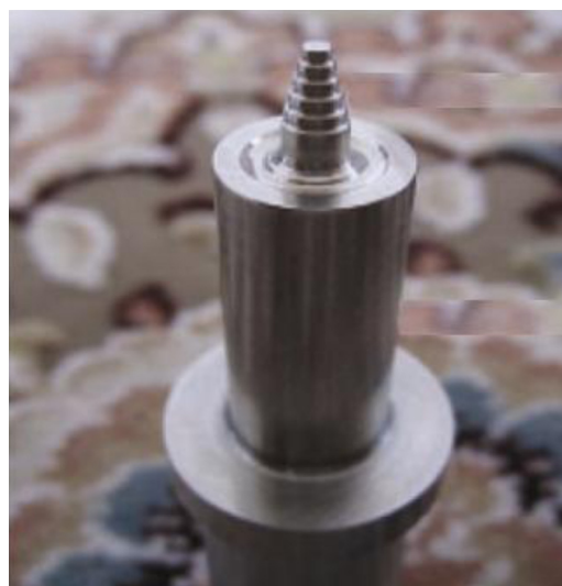
Fig. 3 – Cylindrical-conical grooved pin tool which is used for experiments.
