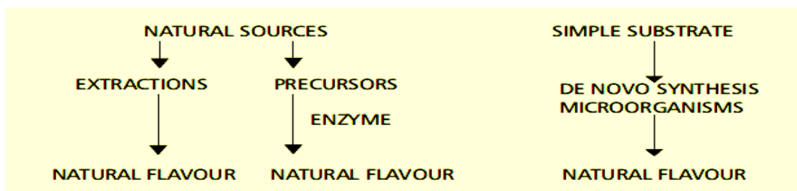
Fig.2. The three pathways for the preparation of 'natural' flavors. The first two involve the extraction of the flavor or precursors from natural sources. The last method is the de novo synthesis of the flavor by microorganisms growing on simple substrates such as glucose and sucrose.
