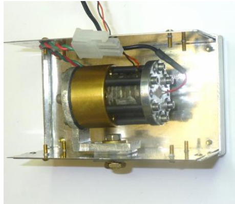
Fig. 1: A PZT stack device mounted in half of a Faraday cage. The Faraday cage sits on the end of a very sensitive torsion balance beam. Visible are the brass disc, the six 2-56 bolts covered with heat shrink for insulation, the PZT discs and aluminium end cap with embedded thermistor.
