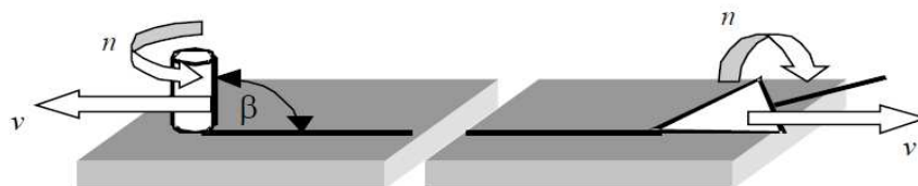
Fig. 34: Principle of quasi-yarn creation
