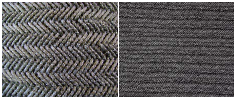
Fig. 21: Examples of braided cloth. Left hand side from 22% carbon fiber co-mingled tows, right hand side from 13% carbon fiber co-mingled tows.
