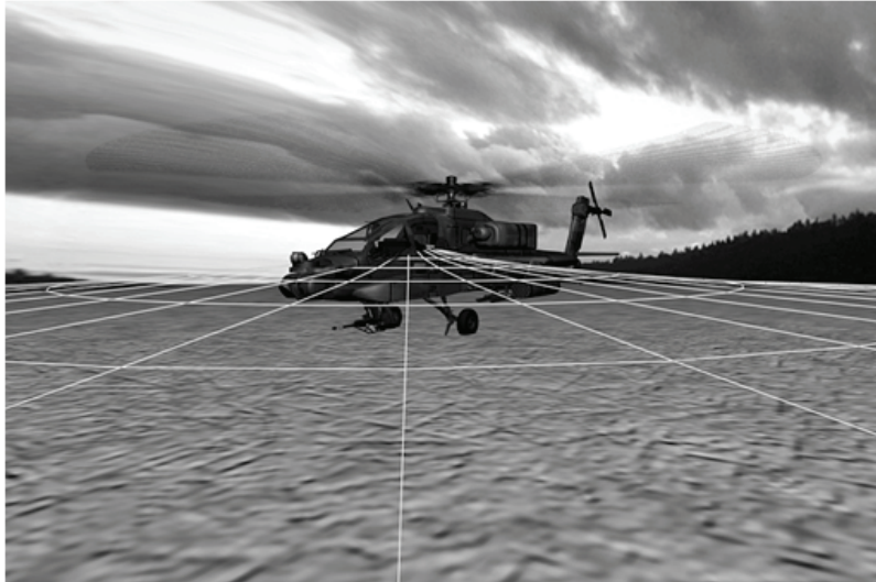
Figure 10-5. Increased separation of I^2 tubes mounted on a HMD exaggerates horizontal, but not vertical perspective. The increased horizontal perspective makes near objects appear closer, as represented by the grid lines, creating a 'crater' illusion. The distant ground appears to level off due to reduced effects of convergence and retinal disparity.
