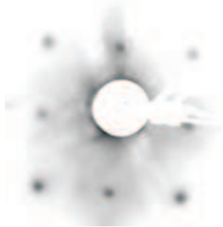
FIG. 11: LEED pattern of \text{Co}_2\text{FeSi}/\text{MgO} , taken at 318 eV primary electron energy. The pattern demonstrates a clear fourfold symmetry.
