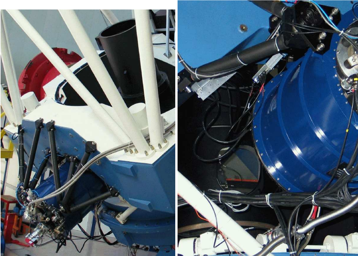
Fig. 16.— The GROND instrument at the 2.2 m telescope. Left: Grand view of the telescope, GROND to the lower left, the light baffle on top of M3 in the middle, and the main electronics rack at the top. Right: Blow-up of the GROND vessel and its various connections. The backside of the cryostat contains the CCC, the turbo-molecular pump, as well as a small emergency pump for rare cases of power outages.
