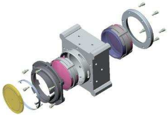
Fig. 9.— Exploded view of the lens mounting block for the 4 collimator lenses in each of the three NIR channels.
