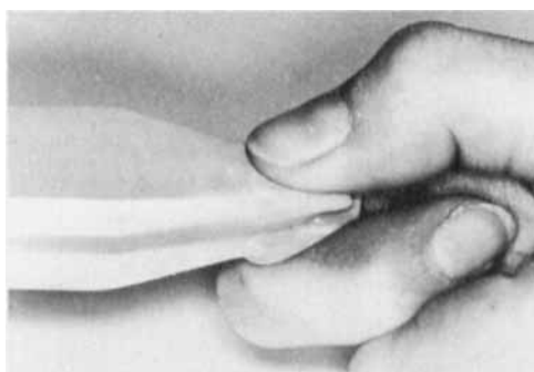
Fig. 2. Measurement of finger-thumb grip with 25 kg fork.
