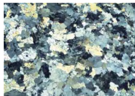
Figure 7: Photomicrograph in cross-polarized light of very compact sub-grain aggregate in Myanma jadeite (section width 10 mm), in which some precursor grains show sutured boundaries.
