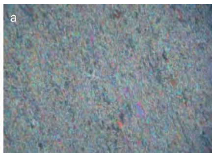
Figure 6: Thin sections showing semi-orientated to preferred orientated jadeite crystals in feitsui from Myanmar: (a) Fine-grained, orientated and compact texture of a near-glassy jade (section width 2.5 mm, cross-polarized light); (b) Semi-orientated grains of intermediate size form a translucent jade (section width 2.5 mm, cross-polarized light).
