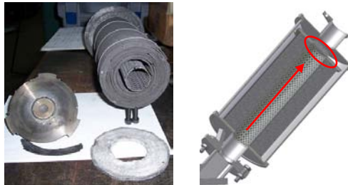
Figure 13: Failure position of prototype 2 after 18.5 hours.
