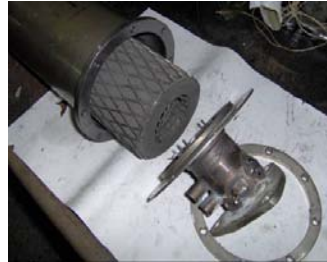
Figure 12: Failure of the perforated tube of Korean 12132 after 21 hours.
