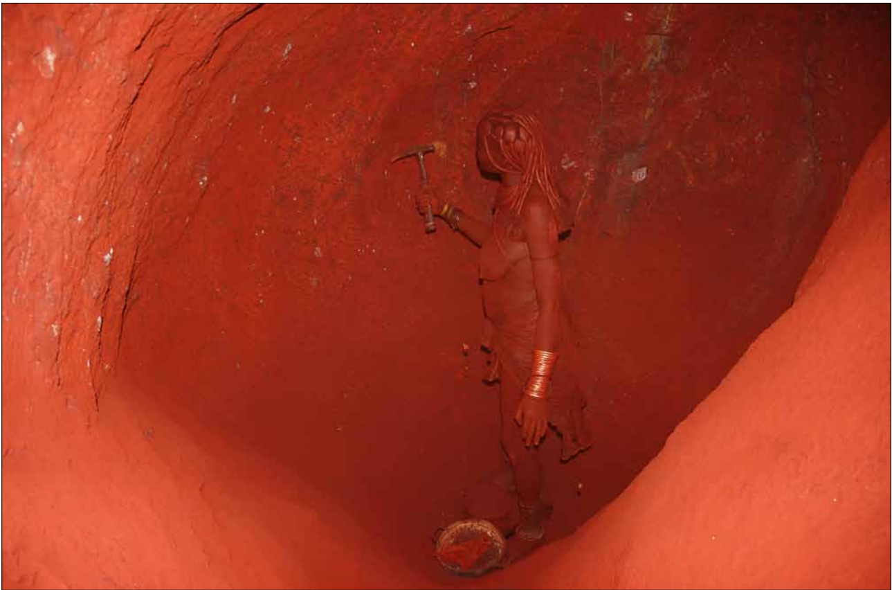
Abb. 8 Female Himba miner, extracting haematite ore in the deepest stope of the mine with a geological hammer borrowed from the author. The stope face has acquired such a smooth, round shape that the extraction of chunks of ore has become extremely difficult without fire-setting.
