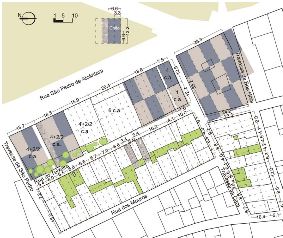
Figure 2: Plan of a section of Bairro Alto, Lisbon, Portugal, showing building measurements. Source: Fabiana Pavel.
