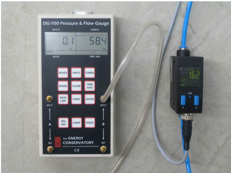
Figure 23 Close up of Festo flow meter and Energy Conservatory DG-700 pressure gauge
