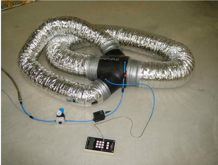
Figure 22 Set up of pressure test rig, showing BTO, duct, pressure regulator, flow meter, valve and manometer.
