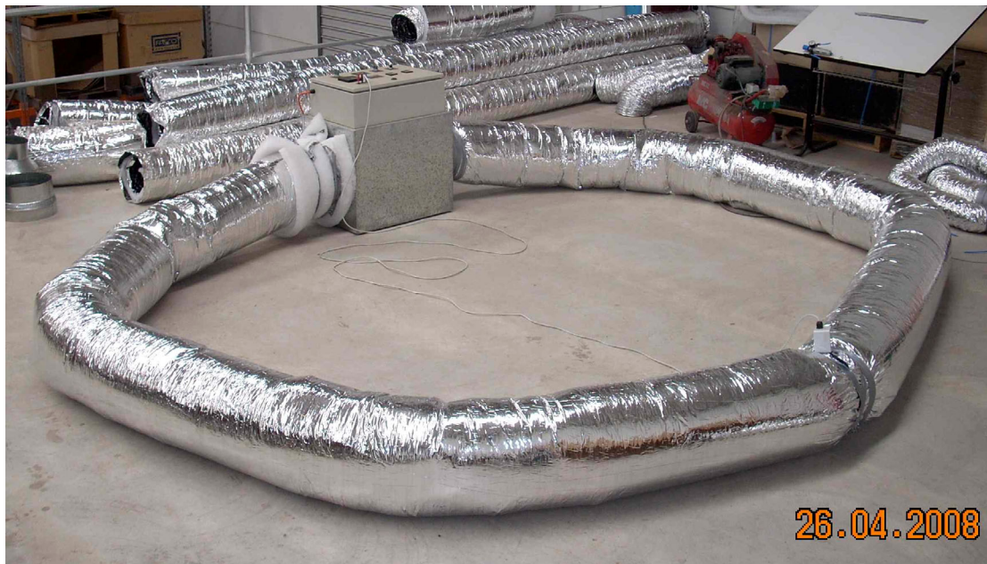
Figure 21 Thermal test rig with 2 lengths of 6 metre flexible duct connected in a “donut” configuration. Heater/fan assembly is the box at the centre.
