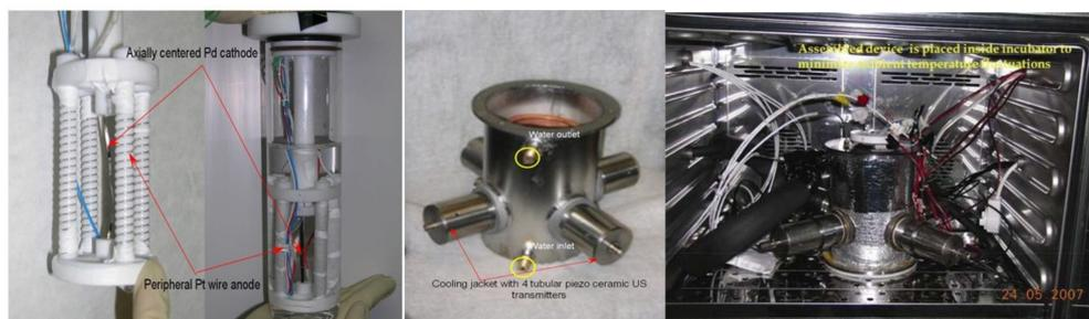
**Figure 2.** Photos of US4 calorimeter; a) anode-cathode (non-tension version) assembly and electrochemical cell, b) SS chamber, c) assembled calorimeter in incubator cabinet.
