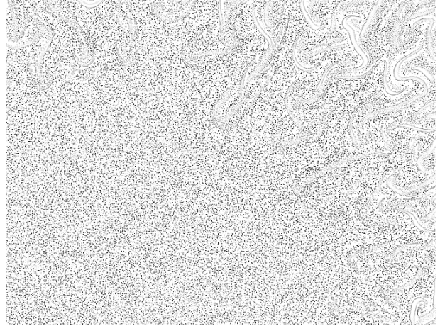
Figure 6. Processed particle image in Figure 1, after the application of local contrast normalization and DoG filter.
