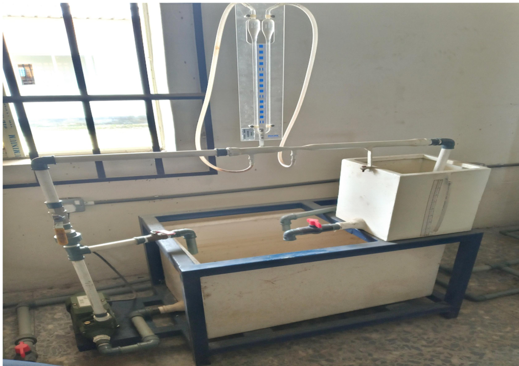
Figure 1.3: The AKSU Venturimeter flow rig being integrated alongside other fluid mechanics equipment in the fluid mechanics laboratory in AKSU, Nigeria (Ekong, G. I. 2020)
