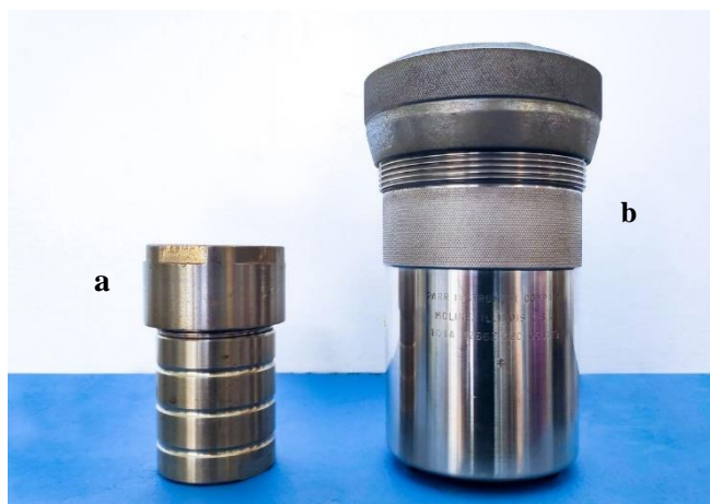
Figure 2. Images of the (a) HAR and (b) POCV used for hydrothermal carbonization
