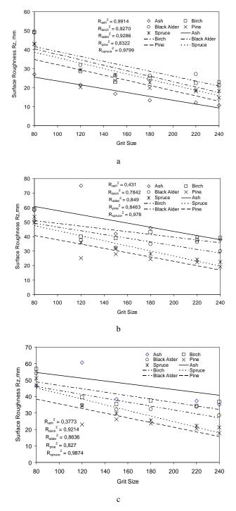
Fig. 2. Surface roughness dependence on the grit size and wood species: a – along the grain; b – across the grain; c – in the angle of 45°
