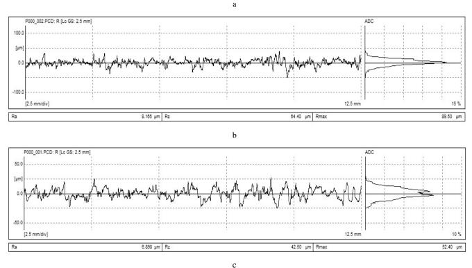
Fig. 1. Typical surface roughness  $R_z$  profiles of birch wood: a – along the wood grain; b – across the grain; c – in the angle of 45°
