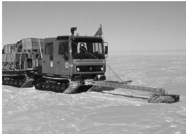
Fig. 5 Ground penetrating radar mounted on a 7-m long metal rod in front of the BERCO TL6 tractor, East Antarctica. The radar transducer is installed inside the rubber inner tube at the right end of the rod, which is connected with a cable to the digital control unit installed in the tractor cabin.
