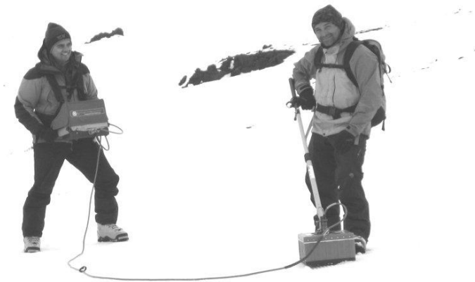
Fig. 4 Ground Penetrating Radar used on Volcán Mocho-Choshuenco, Chilean Lake District. The operator on the left has the digital control unit, while the person on the right carries the transducer.
