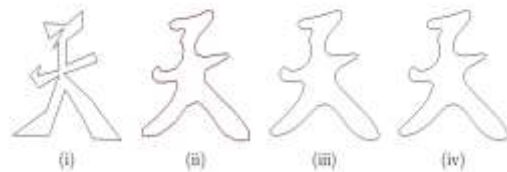
Figure 2: (i) Initial closed polygon. After applying 1st, 2nd and 3rd subdivision steps, we get (ii), (iii) and (iv).
