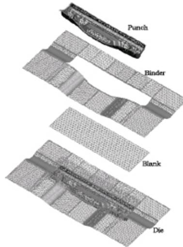
Fig.4 FEM models of tools and blank for simulation
