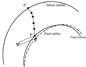
Fig. 2 Nodes move on trimming line in the optimization
