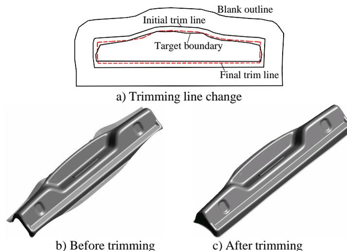
Fig.5 Blank outline, target boundary and part after of the calculation of the cut contour
