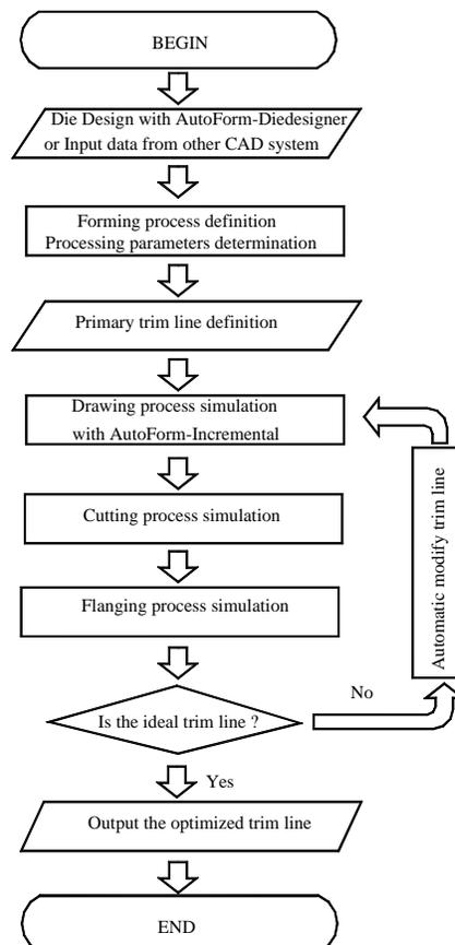
Fig.1 Flow chart of trimming line optimum by FEM
