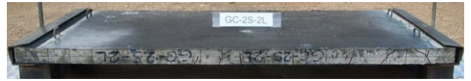
Fig. 18. Crack pattern and deformed shape of Specimen GC-2S-2L under second explosion (Image by G. Tanapornraweekit)
