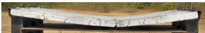
Fig. 5. Deflected shape and crack pattern of Specimen C4 (Image by G. Tanapornraweekit)
