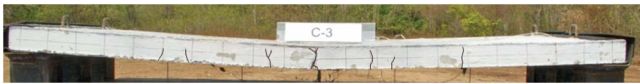
Fig. 4. Deflected shape and crack pattern of Specimen C3 (Image by G. Tanapornraweekit)
