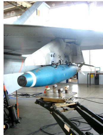
(c) Dummy bomb connected to the left wing.
