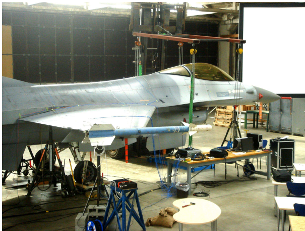
(b) Dummy missile mounted at the right wing tip.
