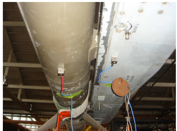
(e) Potential nonlinear connection instrumented on both sides.
