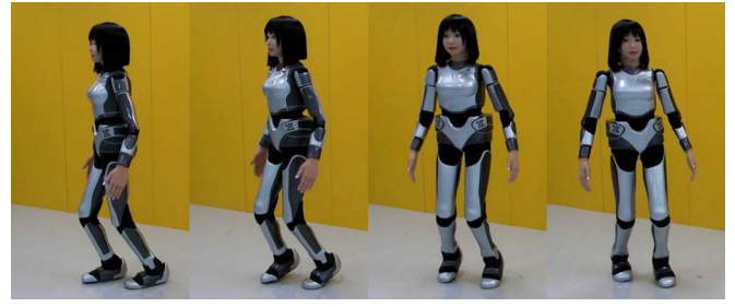
Fig. 2. HRP-4C turning on its toes. Total motion period: 3.0[s], toe support period: 1.2[s], turning period: 1.05[s], and maximum angle of toe joint: 30.0[deg].
