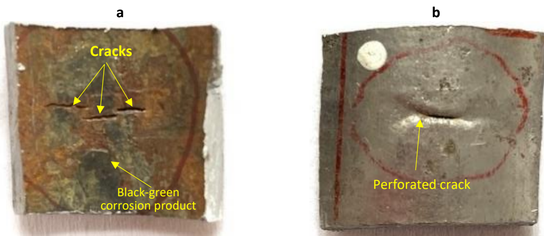
Figure 4. Cracks on a - the inner surface and b - the outer surface
