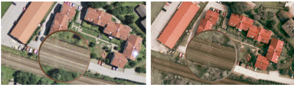
Figure 6: Color image segment from aerial film (left) with a GSD of 15 cm, obtained from a 12.5 \mu m scan. The UltraCam-image has a GSD of 16 cm (right). The inserts are 2x enlarged and have a diameter of 150 pixels. Note the definition of the railroad track.
