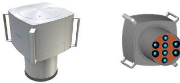
Figure 6: Overview of the UltraCam D large format digital aerial camera. A set of 8 optical cones exists holding a total of 13 CCD arrays to assemble a large format digital image in RGB-color and near infrared NIR. Multiple area array CCDs collect pixels. Each CCD array feeds signals into their own compact and proprietary electronics setup and data path. For dimensions and weight see Table 1.
