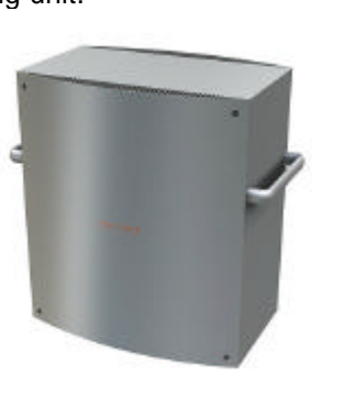
Figure 7: The UltraCam-D/SCU storage and computing unit for distributed parallel UltraCam data collection and on board processing. A total of 15 CPUs and 30 (mobile) hard disks collect and process up to 1 Tbyte of data at a minimum interval of 0.75 seconds per image take. For dimensions and weight see Table 1.
