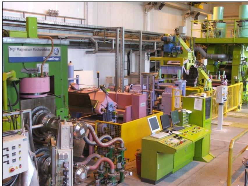
**Fig. 1:** Photograph of the twin-roll caster (in the front) and the four high quarto reversing mill (in the back) at the Institute of Metal Forming, TU Bergakademie Freiberg
