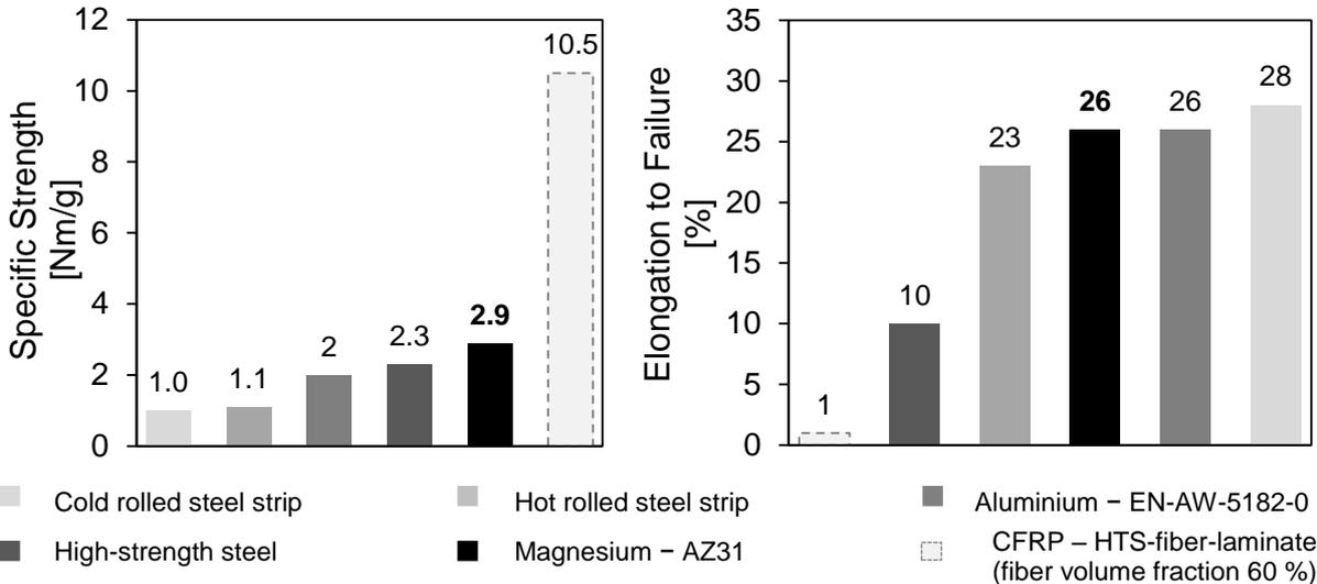
**Fig. 6:** Comparison of specific strength ( $R_m/\rho$ ) and elongation of several lightweight materials used preferentially in the automotive industry [5, 9-11]
