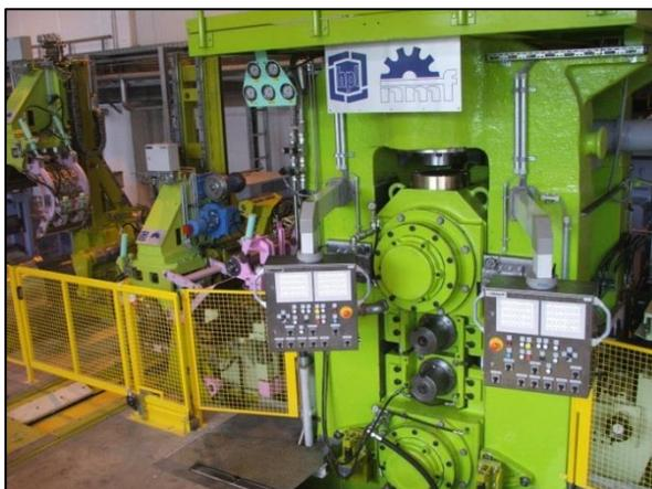
**Fig. 2:** Photograph of the four high quarto reversing mill
