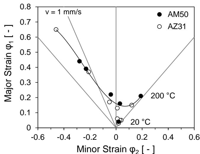
**Fig. 5:** Forming limit diagram of AZ31 and AM50 at different temperatures
