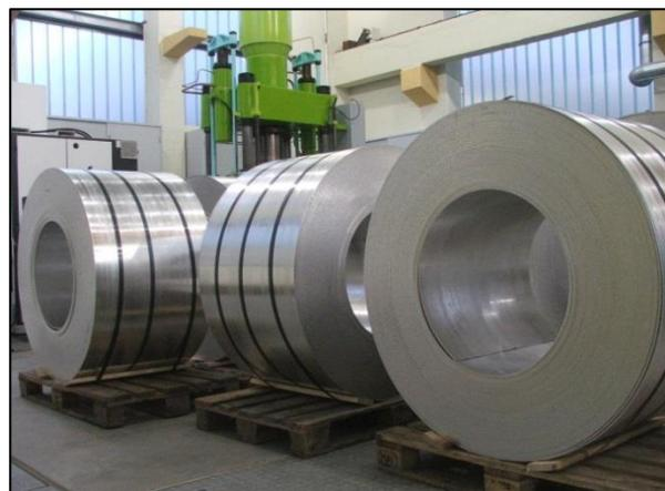
**Fig. 3:** Photograph of the twin-roll cast and hot rolled Mg coils
