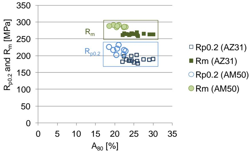
**Fig. 4:** Mechanical properties of the final rolled and annealed strips with a thickness of 1.5 mm at room temperature (longitudinal direction)
