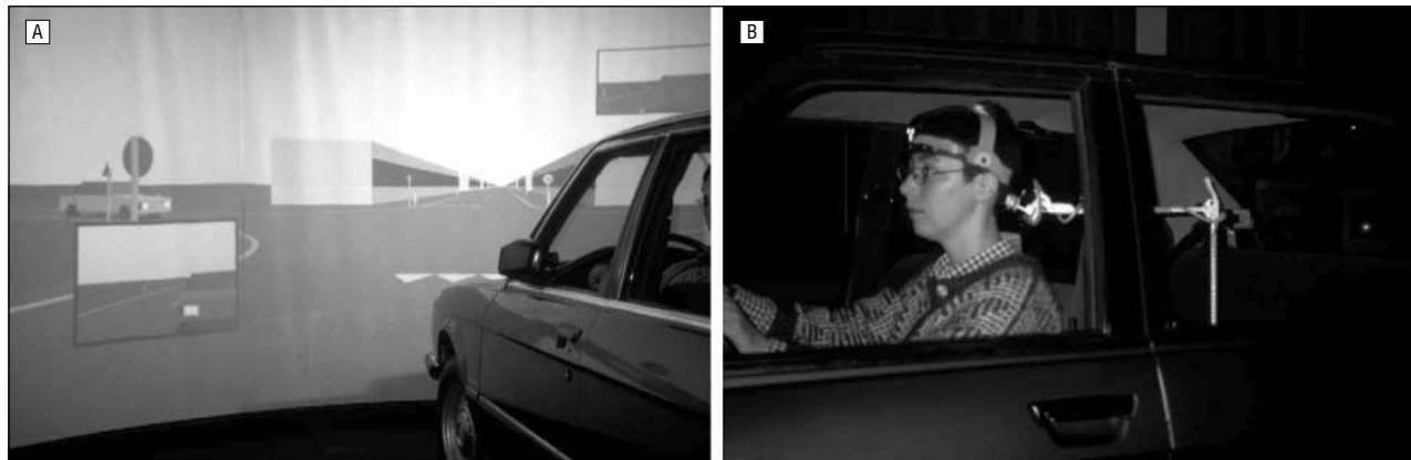
Figure 2. A, The driving simulator. A modified car was positioned in front of a 165° × 45° projection screen. Roads, intersections, traffic lights and signs, buildings, sideview and rearview mirrors of the car, and other vehicles were projected on the screen. B, A head tracker monitored subjects' head movements while they were driving.
