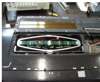
Fig.18. Scale-one APA1000XL-based active flap on Helicopter blade
