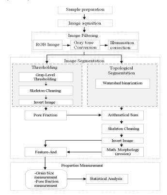
Fig. 1 Block diagram depicting the imageJ analysis procedure adapted from [25].
