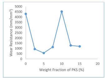
Fig. 5 Effect of concentration of PKS (wt%) on the wear resistance (mm/mm<sup>3</sup>) of AA6063 matrix composites during sliding wear test
