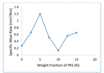
Fig. 3 Effect of concentration of PKS (wt%) on the specific wear rate (mm<sup>3</sup>/Nm) of AA6063 matrix composites during sliding wear test
