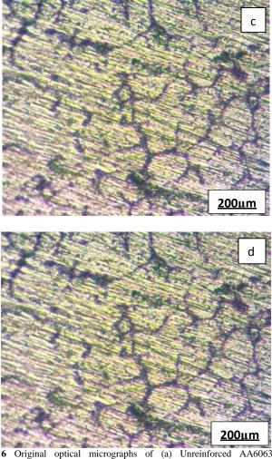
**Fig. 6** Original optical micrographs of (a) Unreinforced AA6063, (b) AA6063/5wt%PKS, (c) A6063/7.5wt%PKS and (d) AA6063/15wt%PKS Composites at 640× magnification
