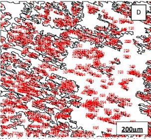
**Fig. 10** Map drawing of the particle area distribution of black and white threshold (using Analyse tool) for (a) Unreinforced AA6063, (b) AA6063/5wt%PKS, (c) A6063/7.5wt%PKS and (d) AA6063/15wt%PKS Composites
