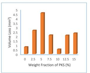
Fig. 2 Effect of concentration of PKS (wt%) on the volume loss (mm<sup>3</sup>) of AA6063 matrix composites during sliding wear test
