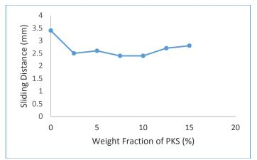
Fig. 4 Effect of concentration of PKS (wt%) on the sliding distance (mm) covered during sliding wear test
