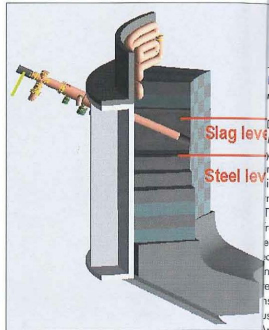
● Figure 1 KT injection system
