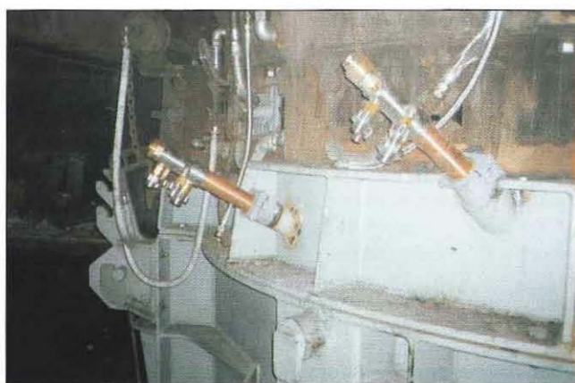
● Figure 5 External view of EAF showing both types of lance
