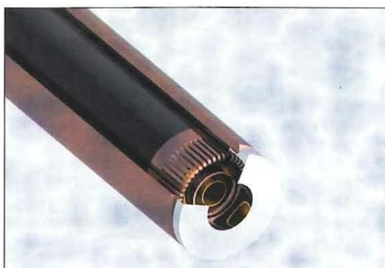
● Figure 4 Cut-away view of cooled KT body (same for oxygen and carbon lances)
