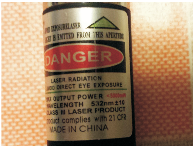
Figure 6: Safety label of Laser 3 does not mention IR emission; the reference to CFR 21 is incorrect
