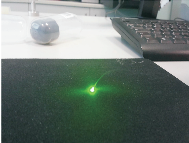
Figure 3: Ignition of rubber after 4 s irradiation with Laser 3
