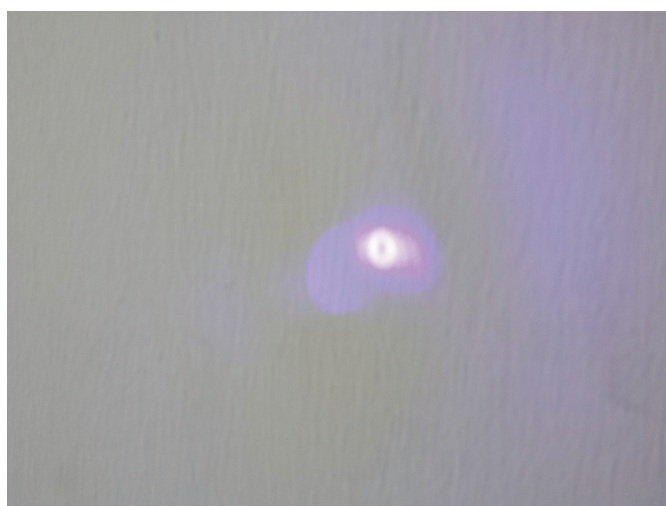
Figure 4: Structure of the broadened spot in laser 4 at 50 cm
