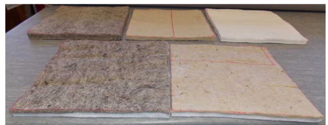
Fig. 17. Samples made of recycled PET tested in [93].
