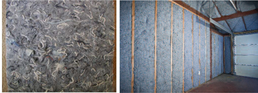
Fig. 18. Panel made of recycled cotton (left) and denim (right) [94,95].
