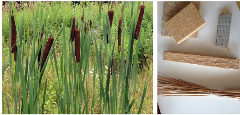
Fig. 5. Cattail plant (left) and cattail fiber panels [61] (right).
