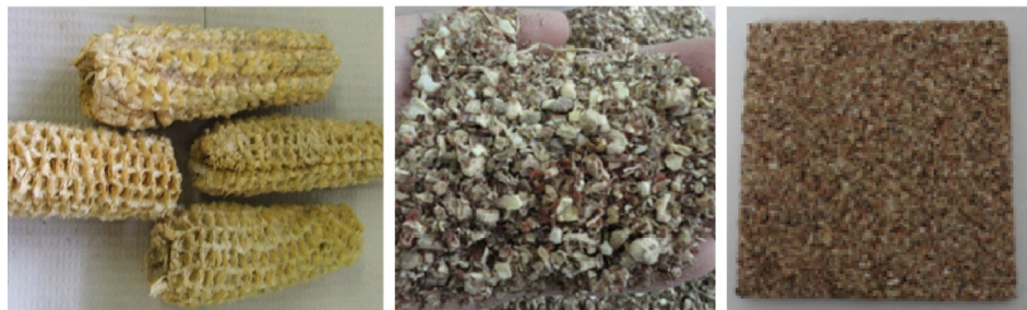
Fig. 6. Corn cob. Raw (left), ground (middle) and panel (right) [63,65].
