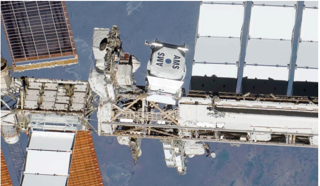
Figure 3. The AMS-02 experiment was installed in May 2011 on the main truss of the International Space Station.
