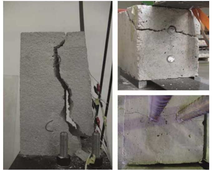
Figure 8. Observed splitting-related failures in EBR specimens.
