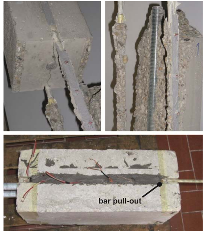
Figure 12. Splitting-related (top) and pullout (bottom) failures in NSM specimens.
