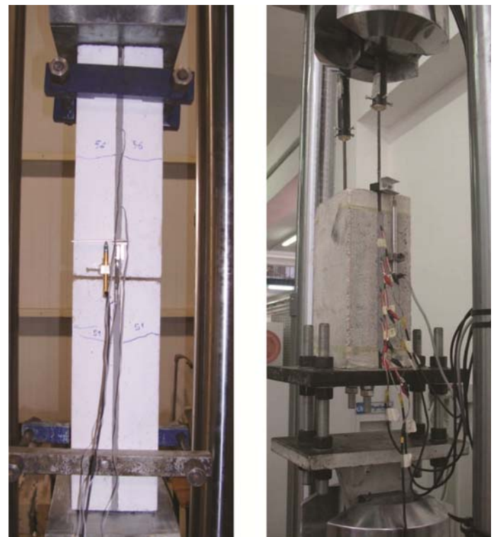
Figure 6. Example of setups used for DS (left) and SS (right) tests on NSM systems.
