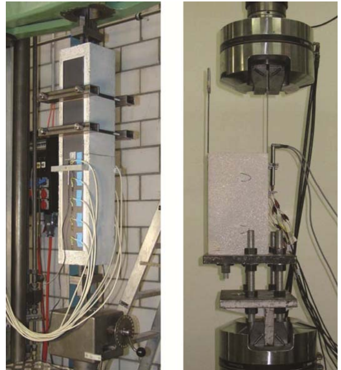
Figure 5. Example of setups used for DS (left) and SS (right) tests on EBR systems.
