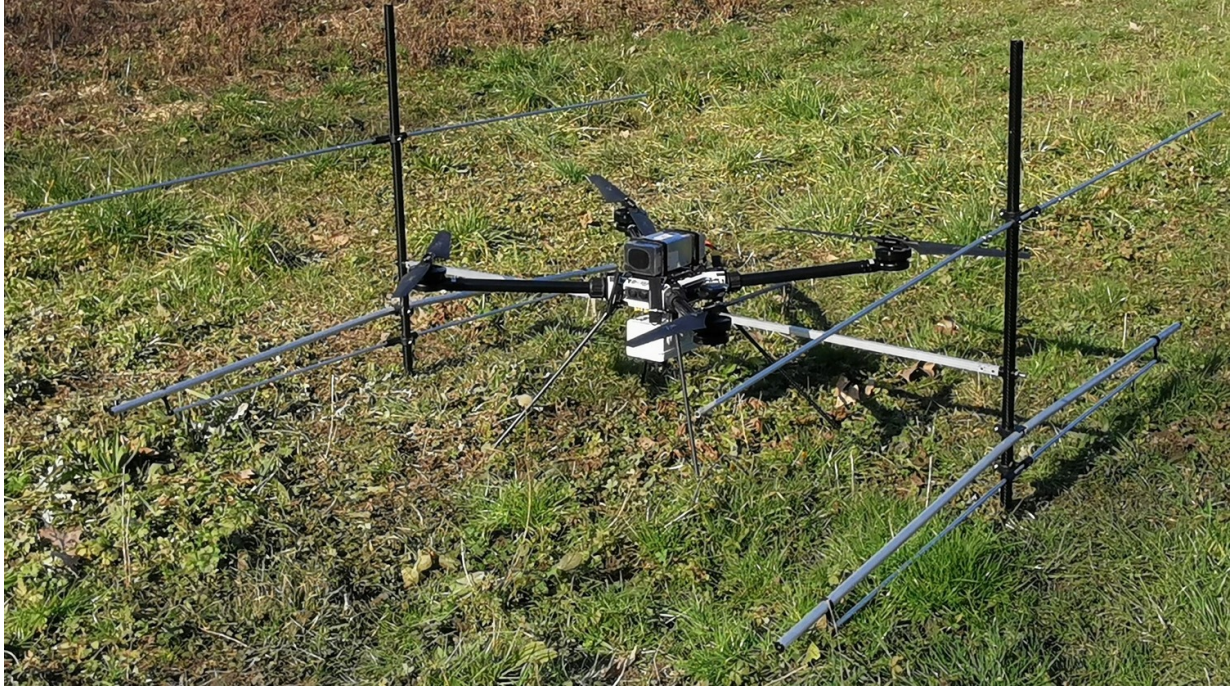
Figure 1: The FlyRadar instrument. The radar's GPS is fixed to the drone's battery in the center. A GoPro camera was added to film the ground.
