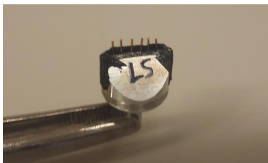
Figure 3.9. Microreactors capillary sections mounted perpendicularly on pin-type aluminium stub using double face epoxy resin tape for high resolution SEM imaging.
