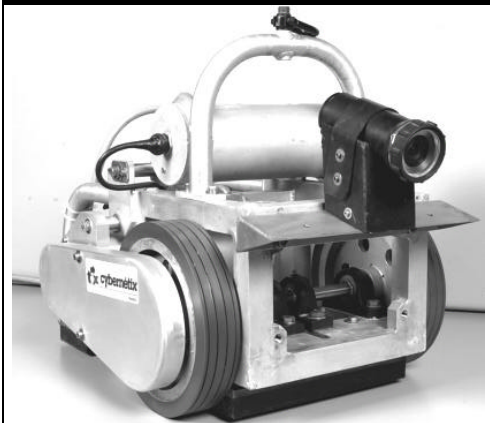
Fig.5: OCTOPUS for underwater Inspection equipped with camera
