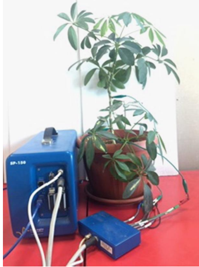
Figure 16.2 Impedance measurement of Schefflera Arboricola using a Biologic SP150 station.
