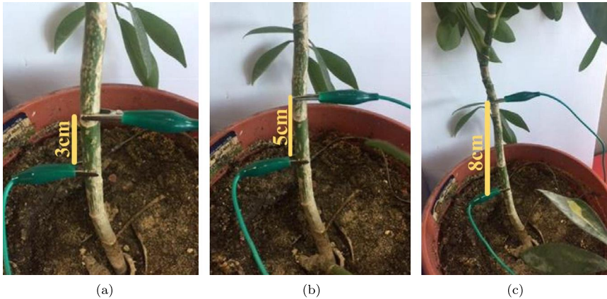
Figure 16.5 Experimental setup for three different interelectrode positions. (a) Position 1. (b) Position 2. (c) Position 3.
