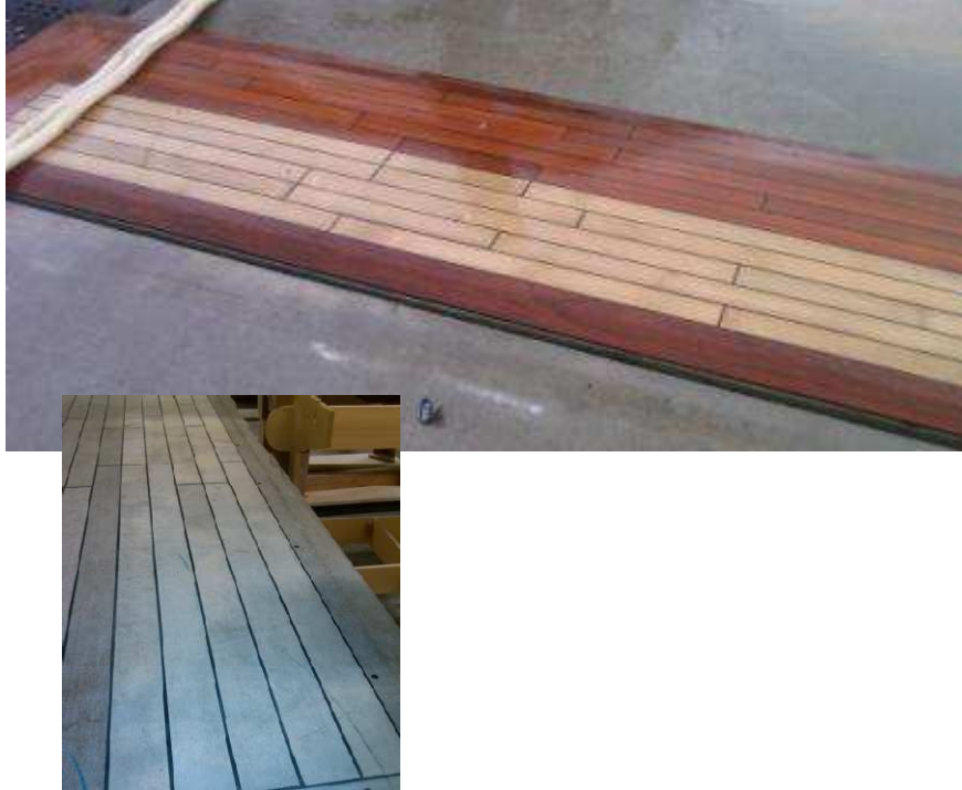
Figure 6 and 7: in situ comparison between Burmese Teak and vertical grain acetylated Accoya Alder. Source: Westport shipyard, Port Angeles, WA, USA.
