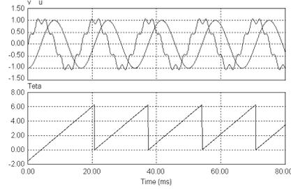
Figure 4- Single-phase PLL: Distorted input voltage, PLL quadrature sinusoid and its cyclic argument angle  $\theta$   $[0,2\pi]$ .
