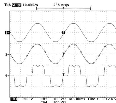
Figure 10 - Active Filter using 3φ-PLL in the selective control: line voltage (1), line current (2) and load current (4).
