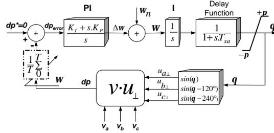
Figure 3 - Three-phase digital PLL using instantaneous inner product of orthogonal functions.
