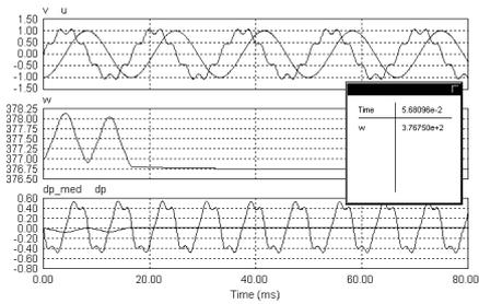
Figure 5- Upper: input and PLL voltages. Middle: PLL frequency. Lower: input/output signals of the average filter.
