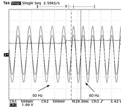
Figure 9 - 3φ-PLL action during a frequency step from 50 to 60Hz.
