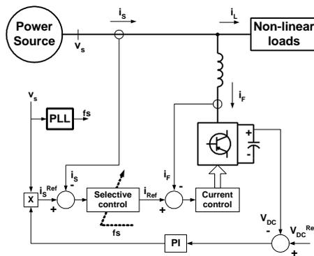
Figure 8 - Diagram of the active power filter using selective harmonic compensation.
