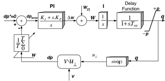
Figure 1 – Generalized 1 $\phi$ -PLL Model.
