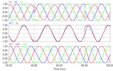
Figure 7 - Three-phase unbalanced voltages during a (-2Hz) frequency step and fundamental unitary 3φ-PLL outputs.
