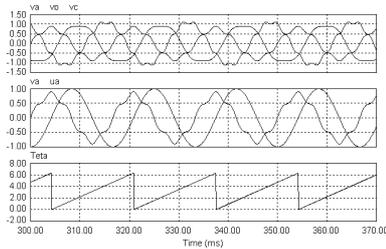
Figure 6 - Three-phase PLL: a study case with distorted and unbalanced input voltages.
