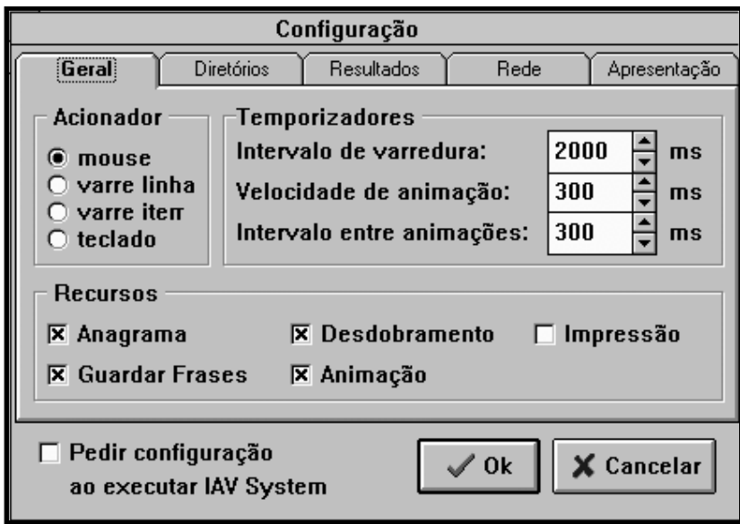
FIGURE 15. Layout of one of the system-configuration screens that permits specifying which parameters (e.g., input devices, scanning strategies and speed) are to be used in order to customize the system to the particular needs of deaf users with serious impairments.
