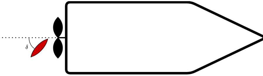
Figure 2.4 : Single rudder and single propeller system.
