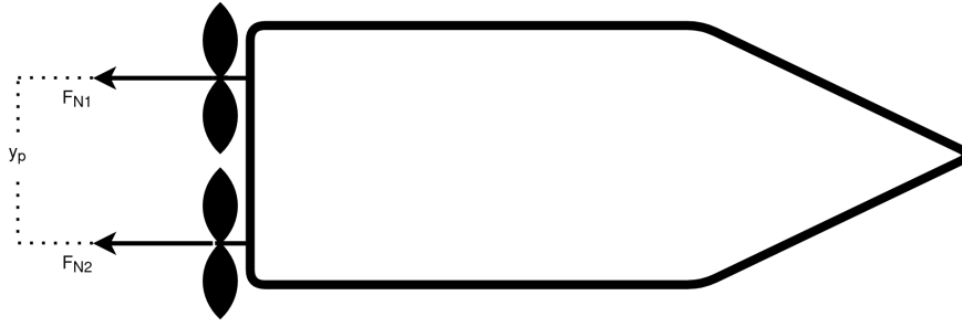
Figure 2.6 : Dual propeller without rudders.
