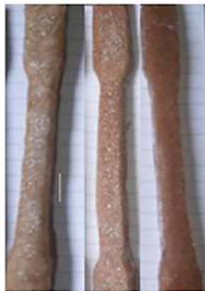
Figure 2: PCLSRC Tensile Test Samples
