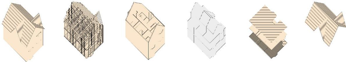
**Figure 1.** Digital model and material layers created by manual on-site survey.
