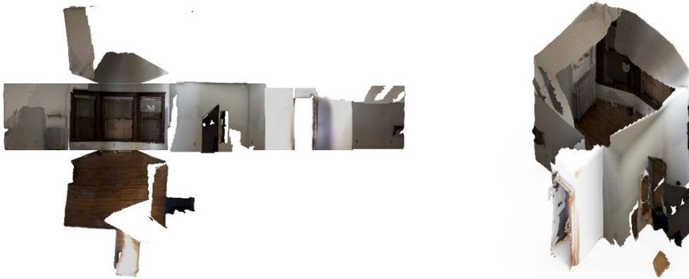
**Figure 3.** (Unrolled) photogrammetry texture map created by digital on-site survey.
