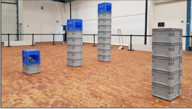
Figure 2: Experimenta order picking setup with with three different removal heights low, medium, high (left) and a storage location (right) (Source: Fraunhofer IML)
