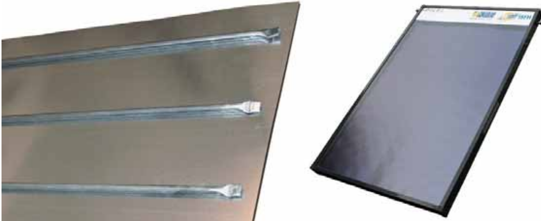
Figure 5: Backside of the aluminum absorber sheet with aluminum heat pipes connected by laser welding (left) and flat plate collector prototype P.1 (right).
