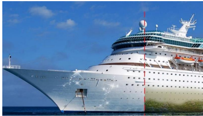
Fig. 2. Developing a special coating with nanotechnology that prevents the growth of marine organisms, such as moss, on the outer layer of the hull of ships by an Iranian knowledge-based company [17]
