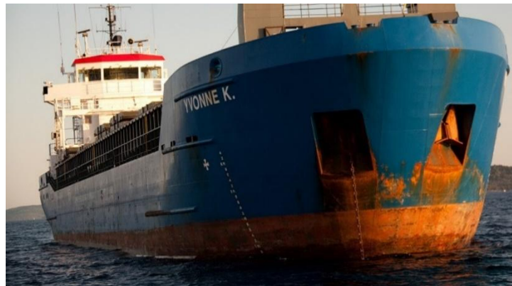
Fig. 3. Corrosion of a ship body [18]
